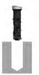
1. Positioning the milling cutter above core hole, check and adjust the length.
