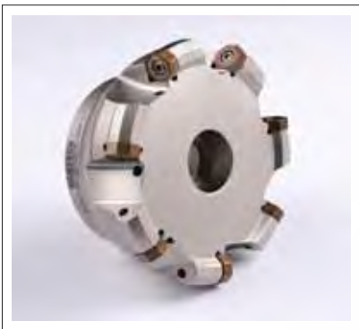
AFM40-ON05-C-45, with 45 degree approach angle, using 16 cutting edge insert with wiper edge. Used in finish milling the flange face of turbocharger casing
